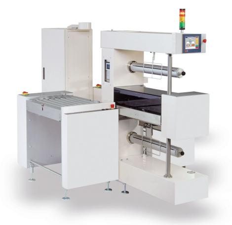
The main cabinet can be pulled out, providing easier accessibility for set-up and maintainance.
