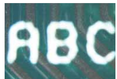
0.7mm text with DotStream Technology™ 1 pass, 26 seconds
