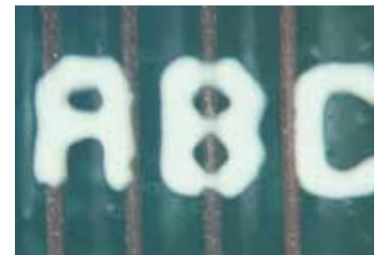
0.7mm text before DotStream Technology™ 2 passes, 58 seconds
