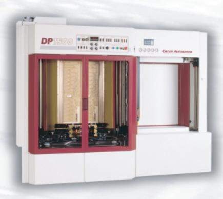
With the addition of the DP-1500-2XL model, ane ven a wider range ofp anel thicknesses and sizes can be coated. The DP-1500-2XL is designed to coat backpanels up to 24" x 36" in size and as thick as 0.400". The unique coating technique of the DP-1500 allows very high traces to be covered with soldermask. Nine mil traces can be covered with adequate thickness on the knee of the trace.
