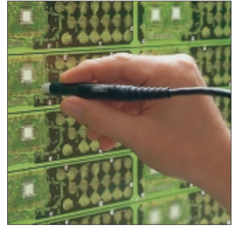
Measurement of the copper thickness in through-holes of printed circuit boards, using the ESL08A probe.
