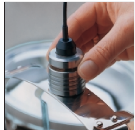
Hand probe Z9NG to measure the coating thickness of, e.g., armatures, printed circuit boards, sheet metal, etc..
