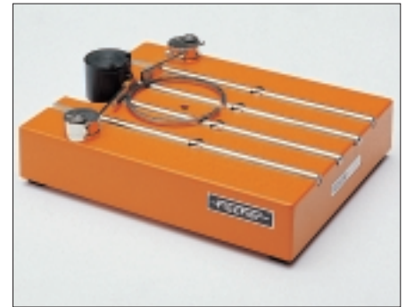
Piston ring measuring table V4EKB4.
