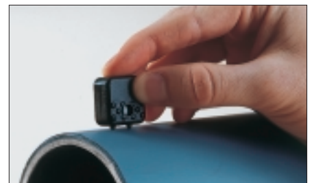
Measurement of synthetic corrosion prevention coatings on pipes using the probe EKB10.
