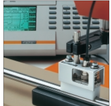
Measurement of the chromium coating on pneumatic cylinders with the probe V2EGA06H mounted in the motorized support stand V12.
