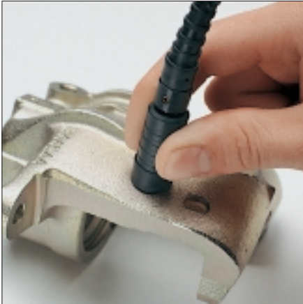
The probe ESD2 is ideal for coating thickness measurements on very rough, electroplated surfaces.
