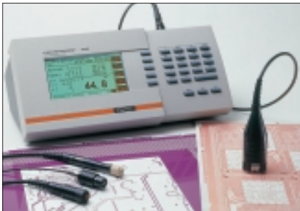
FISCHERSCOPE® MMS® LRP specialty measuring system for quality assurance for pc-boards.
