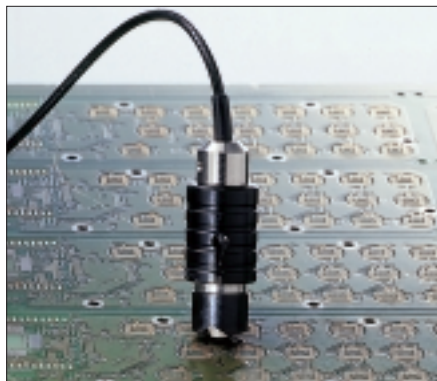
Measurement of the solder resist thickness with the probe ETA3.3.
