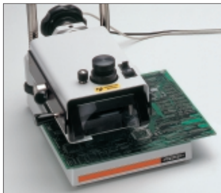
Measurement with the universal measurement stage Z6NG using isotope PM147 and aperture ring \phi 0.63 mm ( \phi 0.02").
