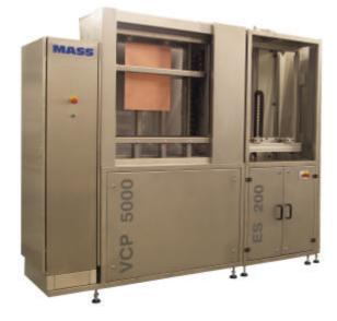
This machine is designed to fill holes in printed circuit boards with conductive or non conductive paste. The hole filling can be performed with through-hole vias and blind vias. The filling of blind holes is possible in a double side mode in one step. The machine is equipped with a glass cover for visual quality control on both panel sides.
